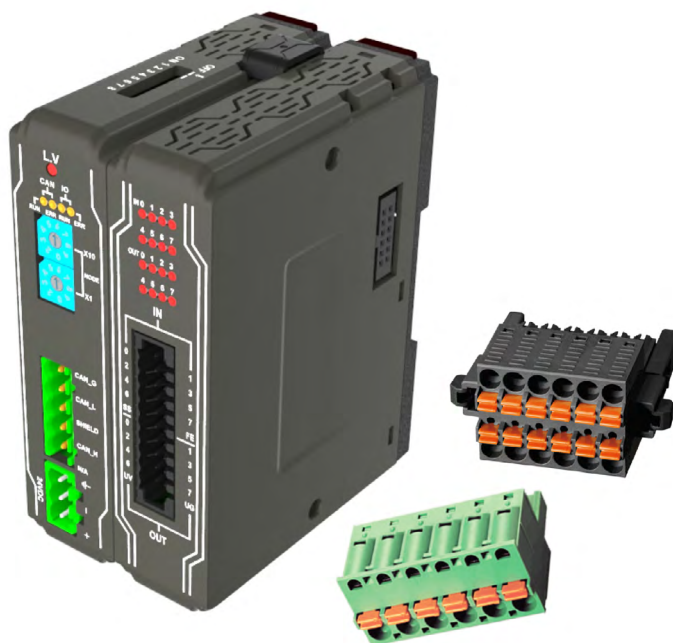
Shown here is an iR-COP CANopen bus coupler with an iR-DM16 module. The bus coupler supports baud rates of 5 kbps to 1Mbps and allows quick node and baud-rate changes. The coupler also allows remote changes to communication settings — and direct EBPro driver support without the need to import code. Shown here (lower right) are plug-in modules that install without a screwdriver; only a flathead screwdriver is needed to remove cables. Up to 16 digital I/O are possible per module (including transistor and relay outputs); up to four analog I/O are possible with 16-bit resolution and configurable voltage ranges including temperature RTD and TC.
